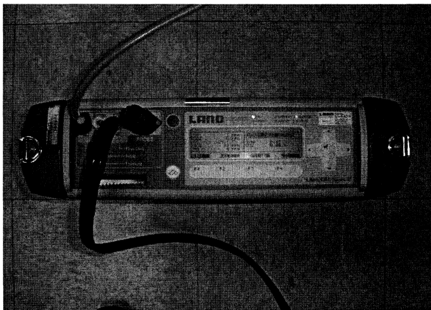
Figure 1.8. LAMCOM gas analyzer for measuring CO and CO 2 .
