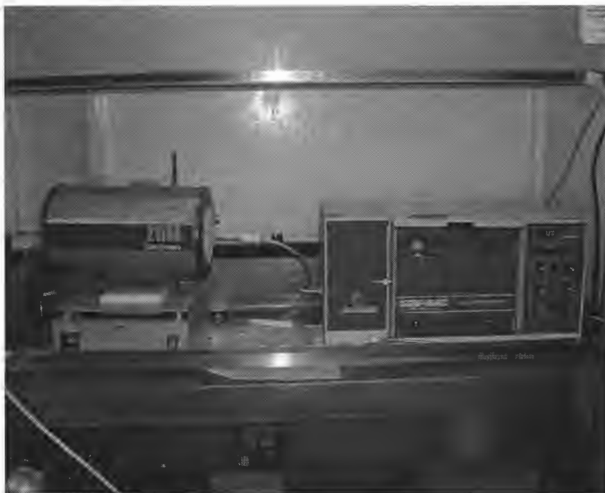
Figure 1.5. Tube Furnace (left) and GC (right) for oxidation of CO and CH 4 .
